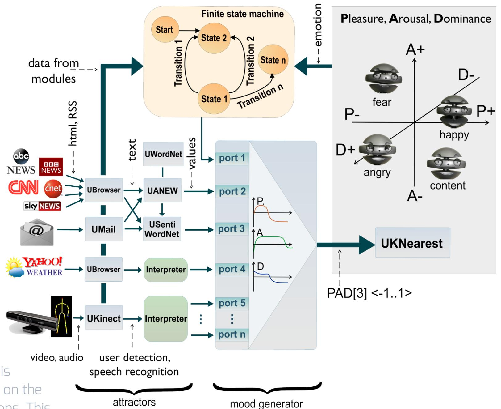
Two emotional systems - Wasabi by Becker Asano and a dynamic PAD-based model of emotion have been adapted to EMYS' control system. Both systems are rooted in dimensional theories of emotion.
