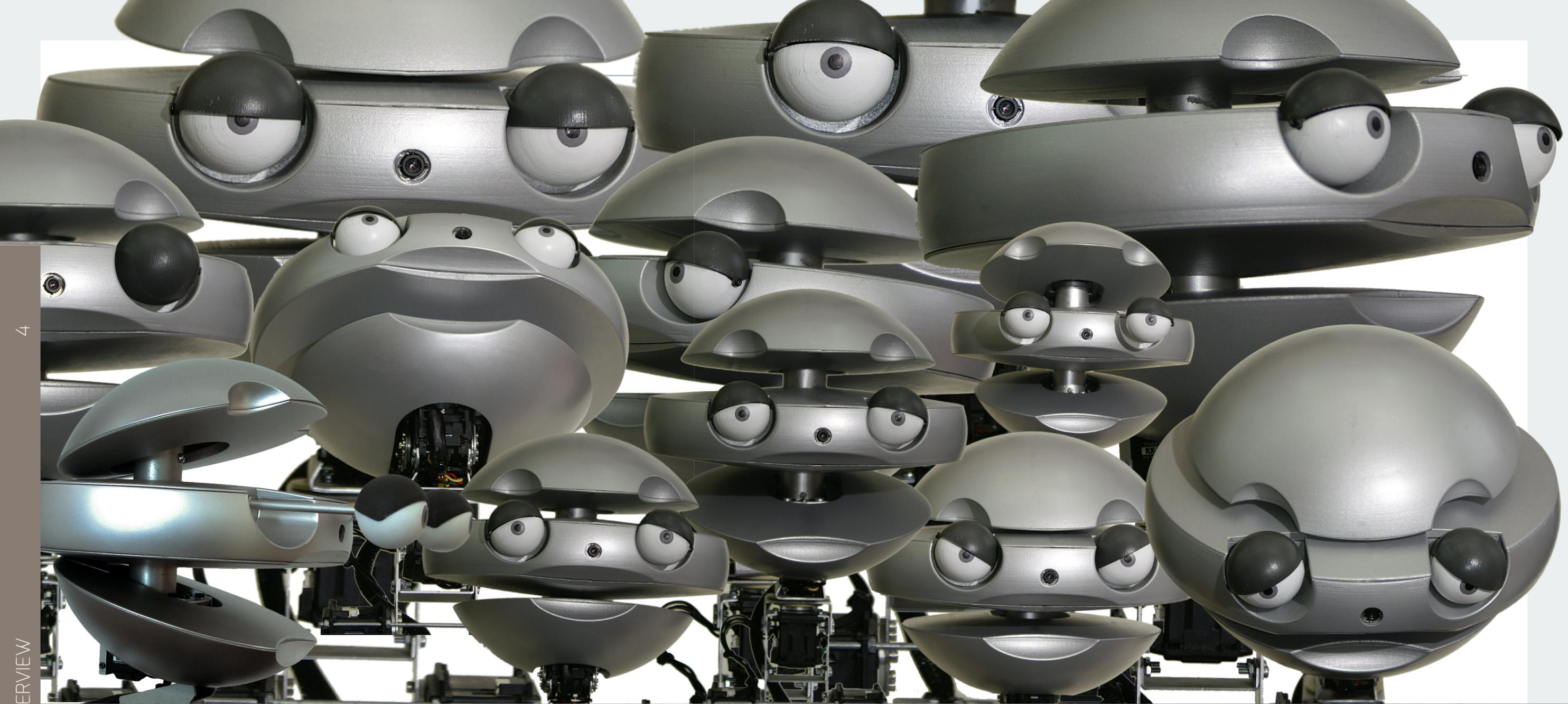
EMYS is an expressive robotic head. It consists of three independent discs of which the upper and lower ones are movable. The robot's popping eyes are situated in the
