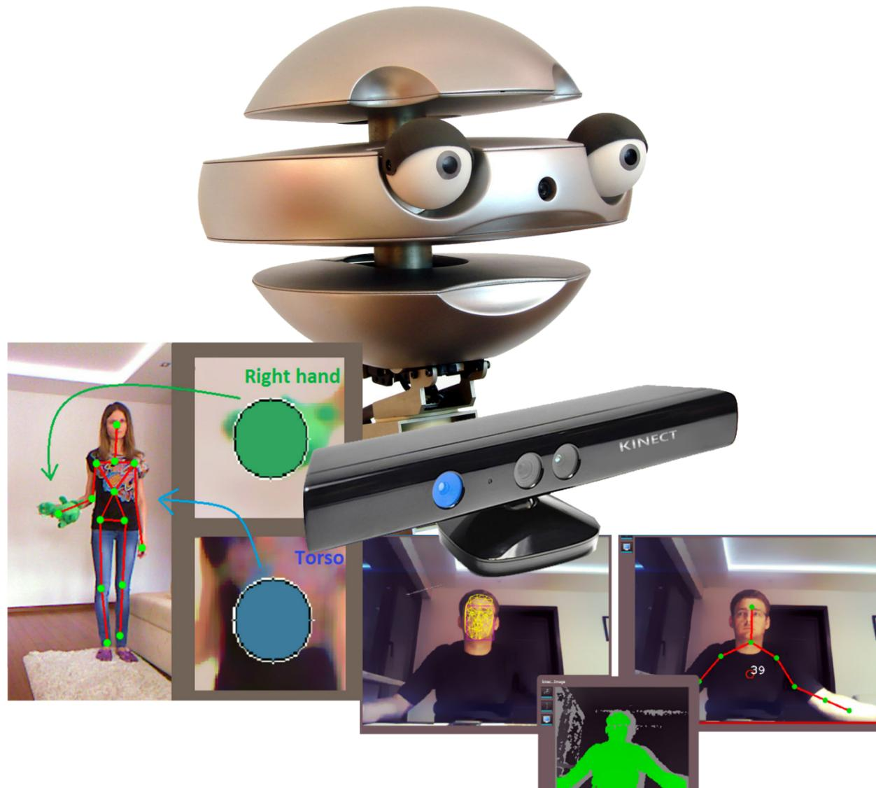
His vision system is comprised of a hi-res camera mounted in his nose and a Microsoft Kinect device playing the role of an advanced motion sensor. It allows him to detect humans as well as provide information on position of particular parts of their bodies. It also provides gesture recognition algorithms, 3D face tracking, and recognition of some facial features.
