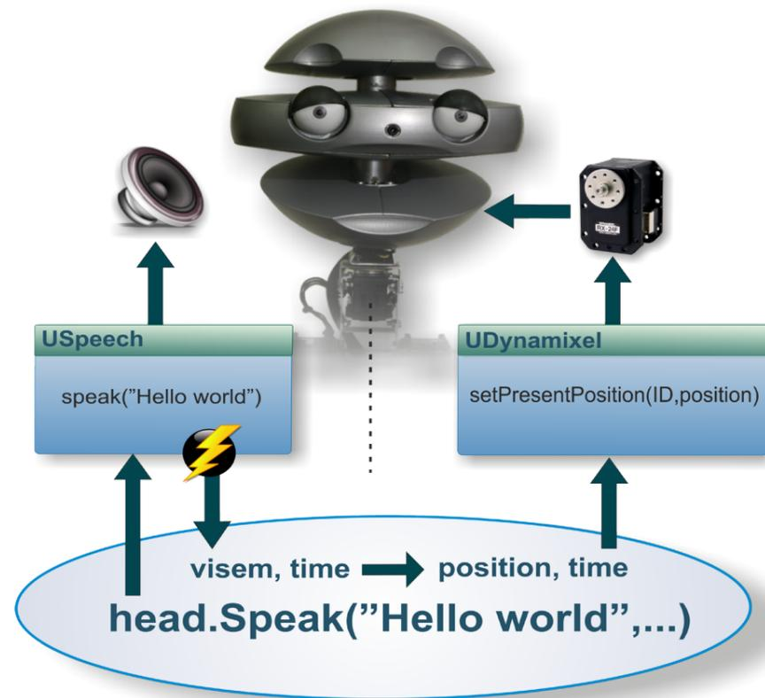
Of particular interest is the orchestration mechanism, built into Urbi, which handles among others the scheduling and parallelization of tasks. Thanks to this feature all the activities of the robot can be synchronized with each other, e.g. movements of joints during head and arm gesticulation, mouth movement with speech, tracking of objects detected in the camera image, etc.
